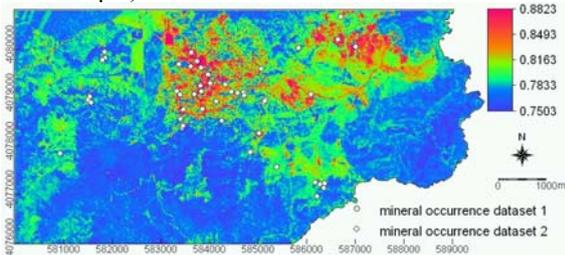
B. Band Ratio 2: arctan transformation on bands 107/109 ( $2.171/2.205\ \mu\text{m}$ ).
